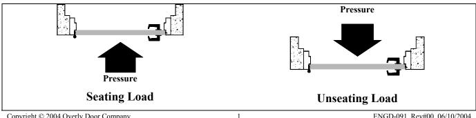
However, if the pressure acts to unseat the door away from the stops, then the hardware must be capable of resisting all loads imposed by the pressure as well as radial and thrust loads. This is an important consideration in the design of both pressure resistant and blast resistant doors, and it has lead to the design of special hinges and locking devices. NB
