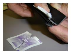
4) Carefully clean the area on the back of the seal that will contact the double faced tape located on the retainer. This should be done using the alcohol wipes provided. Do *not* use mineral spirits or other petroleum cleaning products.
