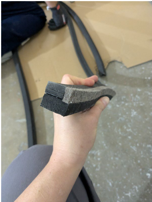
Figure 2 – H-seals prior to installation
