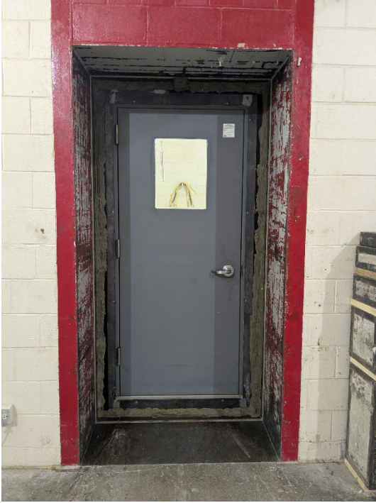
Figure 1 – Specimen mounted in test aperture, as viewed from source room (left) and receive room (right)
