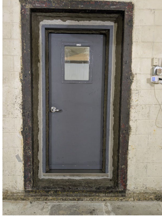
Figure 1 – Specimen mounted in test aperture, as viewed from source room (left) and receive room (right)
