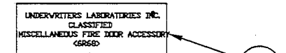
FIRE LABEL TAG MYLOR ADHESIVE BACKED SILVER BACKGROUND WITH BLACK LETTERS LOCATED ON SIDE OF MOUNTING BRACKET
