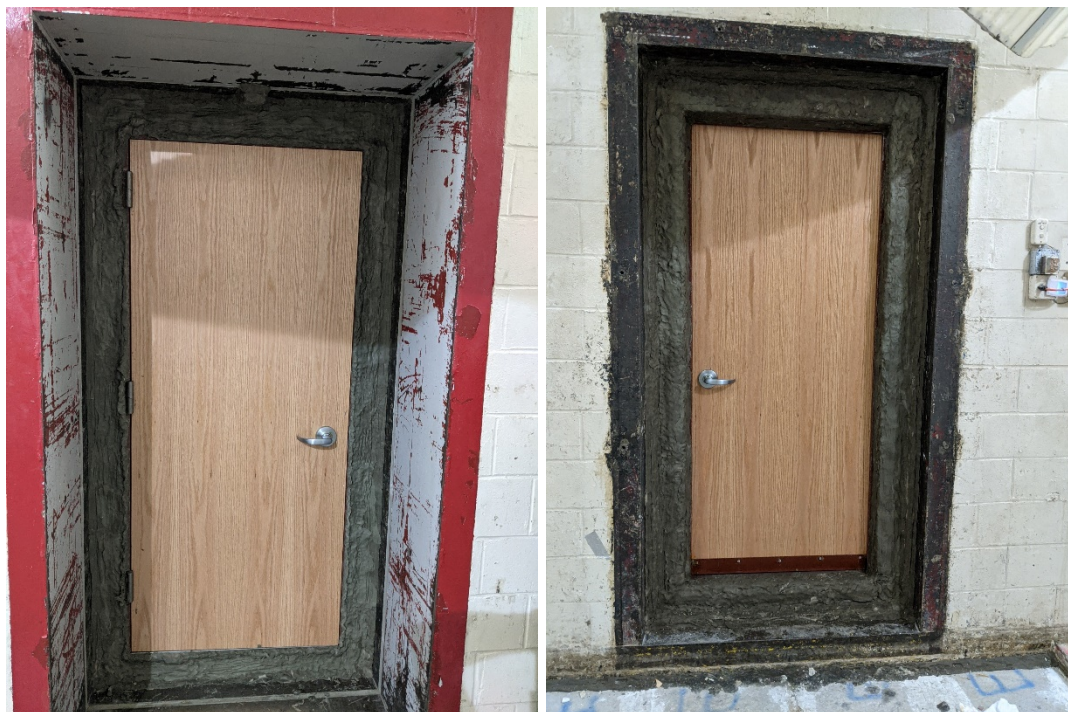
Figure 1 – Specimen mounted in test opening, as viewed from receive room (left) and source room (right)
