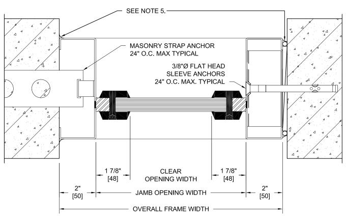
**SHOWING BUILT-IN INSTALLATION** IN MASONRY PARTITION
