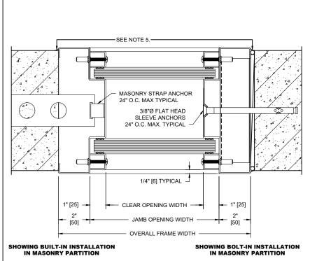
FILL ALL VOIDS IN FRAME [50] 1" [25] 1/2" [12] SBG CLEAR ANNEALED LAMINATED GLASS OR EQUAL OVERALL FRAME WIDTH CLEAR OPENING WIDTH JAMB OPENING WIDTH 4" [102] MINIMUM AIRSPACE 3/4" [19] SBG CLEAR ANNEALED LAMINATED GLASS OR EQUAL 1" [25] 2' PURGE PORT [50] SEE NOTE 4
