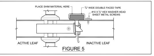
double faced tape as shown in Figure 5. The side closest to the active leaf is left free to allow it to be lifted and shims placed behind. Shims should only be placed in sections where the gasket does not contact active door face.
