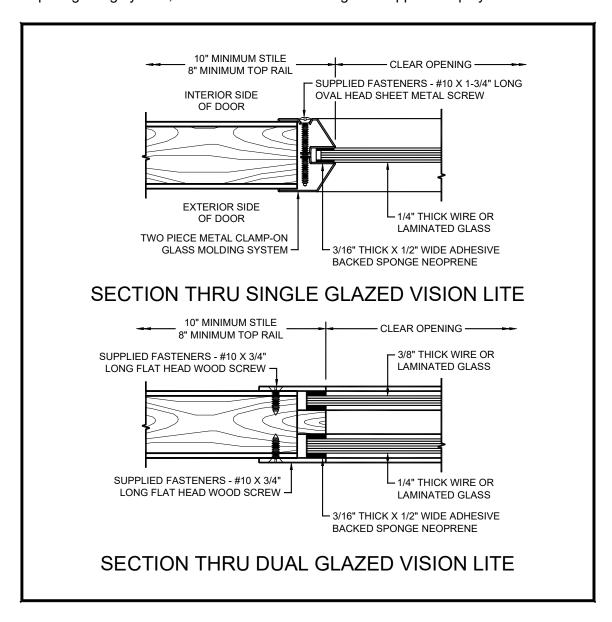
There are several items to consider when placing either vision light systems into an Overly wood door. First is that due to the unique sound-retardant construction required, 10" stile and 8" rail dimensions must be maintained to allow proper preparations in the doors.
