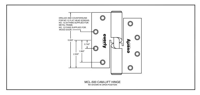
Commercially available level swing ball bearing type hinges are required for sound retardant door models which utilize an automatic type door bottom or raised threshold seal. When this type of hinge is required, Overly recommends that 5" extra heavy hinges be specified to accommodate the increased weight of the wood acoustical door panels.
