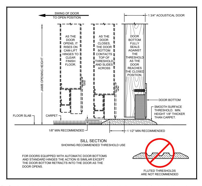
For Overly models that utilize a gasketed threshold to achieve the bottom seal, the threshold must be shimmed so that the bottom of the threshold is at carpet height or finished floor height.
