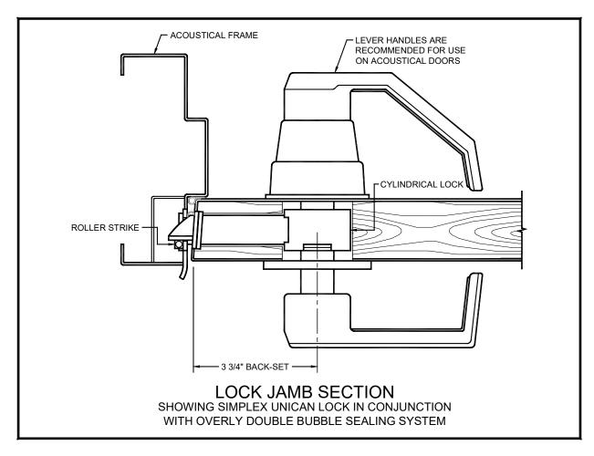
**E. Electric Strikes for single swing openings:** Overly recommends that if electric strikes must be used, sound retardant wood doors equipped with Overly "double bubble" seals be specified. Most electric strikes are too sensitive and bind up when used with compression type seals. The compression seals create pressure between the latch bolt and the gate of the electric strike and will not allow the gate to activate and retract properly.
