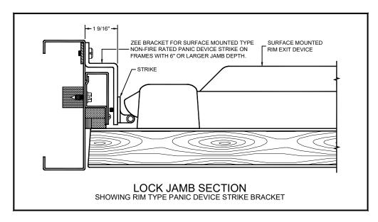
**D.** Rim Type (pairs of doors): For all models of Overly wood doors swinging in pairs using a rim type device for the active leaf of a pair, Overly supplies a roller strike mounting bracket. **Do not mount roller strike directly to the acoustical astragal.**
