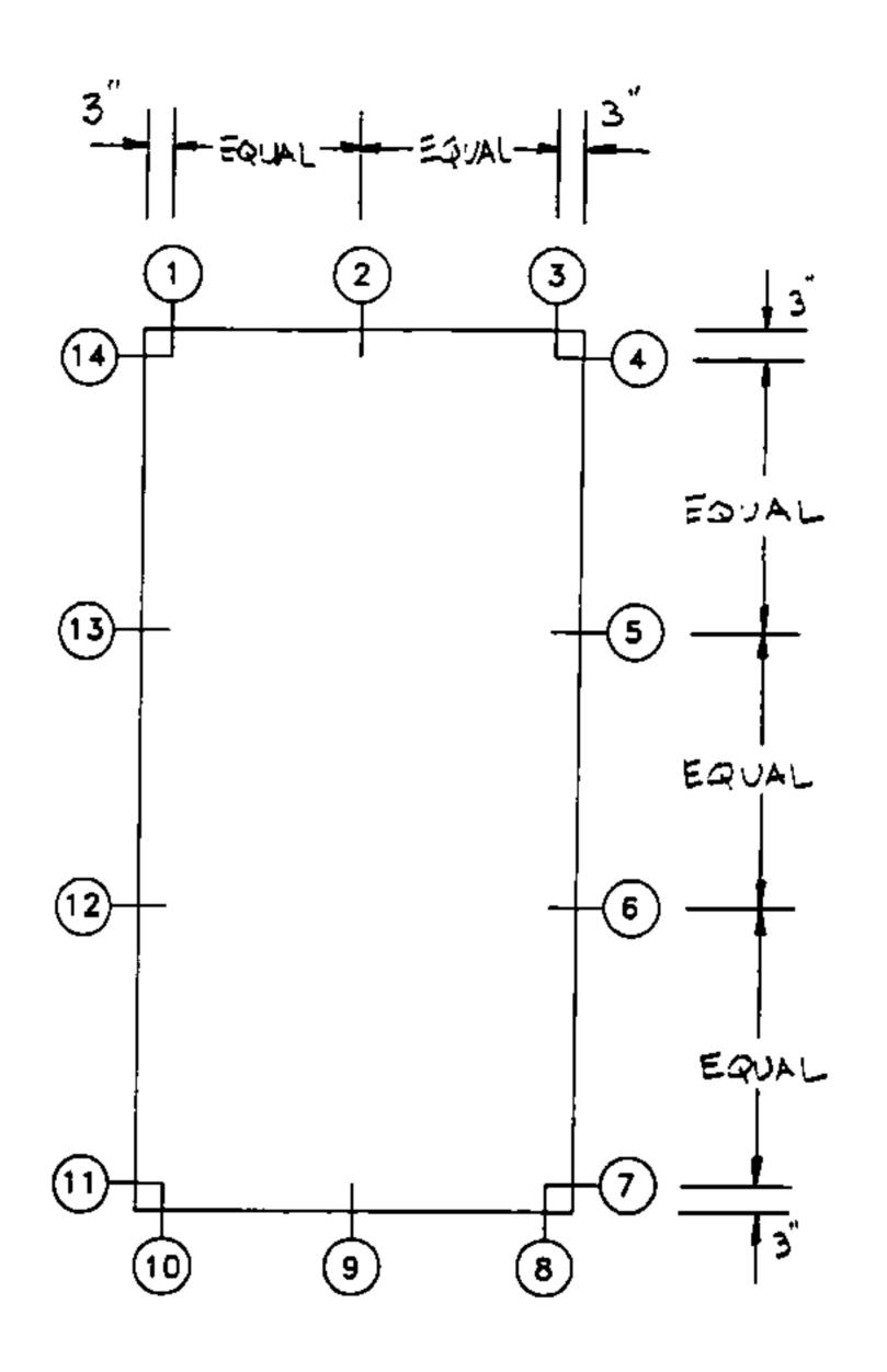
Figure 2 Door Clearance Positions And Door Thickness Positions
