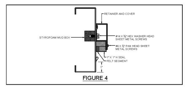
I. After frame has been finish painted, swing door(s) to fully open position. Locate the 1/4" bubble seal package. Measure jamb opening width at head. Cut piece of seal to this length and install on frame rabbet as shown in Figure 4.
