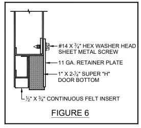
contact the door face, shimming the gasket may be necessary. The gasket is affixed to one side of the steel retainer with a 3/4" wide strip of double faced tape as shown in Figure 6. The side closest to the active leaf is left free to allow it to be lifted and shims placed behind. Shims should only be placed in sections where the gasket does not contact active door face.
