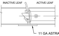
PAIRS OF UL752 BULLET RESISTANT DOORS MUST BE EQUIPPED WITH OVERLAPPING ASTRAGAL BY OVERLY WITH SAME RATING AS DOOR AND FRAME.
